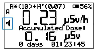
Fig. 33) Acoustic signaling is active
