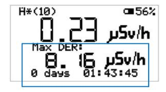
Fig. 8) Mode "dose rate": Display "Max dose rate".
