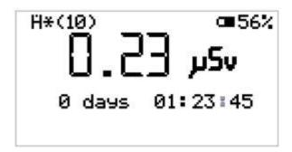
**Fig. 17)** Display in the dose measuring mode μSv.
