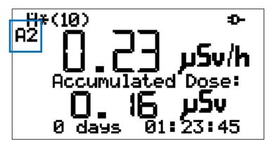
Fig. 29) Alarm threshold A2 is reached at the moment (symbol "A2" flashes)
