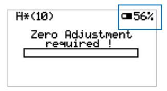
Fig. 19) Display: battery status in percentage
