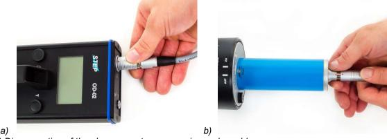
Fig. 23) Disconnection of the plug connectors measuring probe cable.
