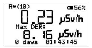
Fig. 16) Display in the measurement mode μSv/h.
