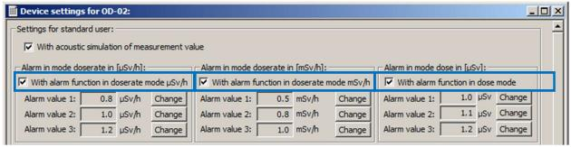
Fig. 25) Setting options for acoustic signaling and alarm thresholds
