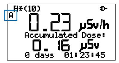
Fig. 28) Alarm threshold(s) activated
