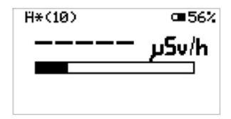
**Fig. 15)** Display in run-in mode for the measuring mode μSv/h.
