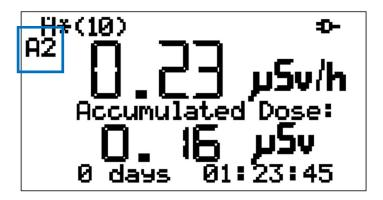
Fig. 30) Alarm threshold A2 has been reached (symbol "A2" remains as a sign)
