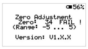
Fig. 13) Zero adjustment beyond the specified range
