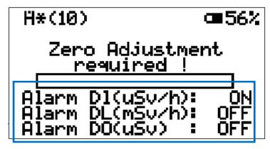
Fig. 26) Start screen with display of active alarm thresholds
