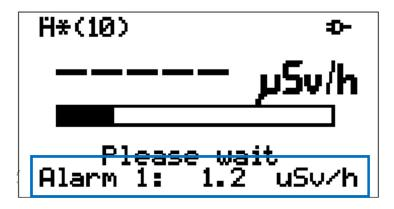
Fig. 27) Alarm threshold displayed when switching over
