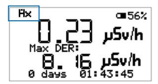
The factor of the applied ionisation chamber of OD-02 / OD-02 Hx amounts to approx. 4.2 fA/µSv·h<sup>-1</sup>. The current generated by the ionisation chamber is transformed into processable voltage by means of the probe electronics. For that purpose, a transimpedance amplifier converts the current via a switchable feedback network into a proportional voltage signal. This voltage signal is scanned in steps of 80 ms in both dose rate modes.
