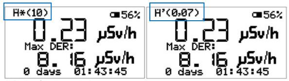
Fig. 9) Display of the dose equivalents
