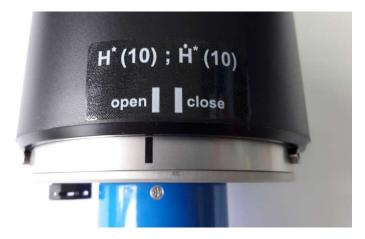
Fig. 14) Interlock of the wall reinforcement cap
